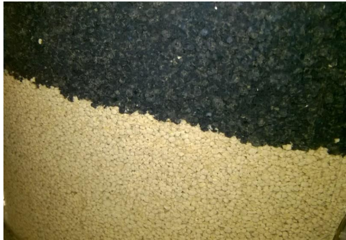
Figure 5.1 – Unselected granules (dark) at the top, from Unicer digester in the beginning of operation and acidogenic selected granules (creamy white) on bottom.
