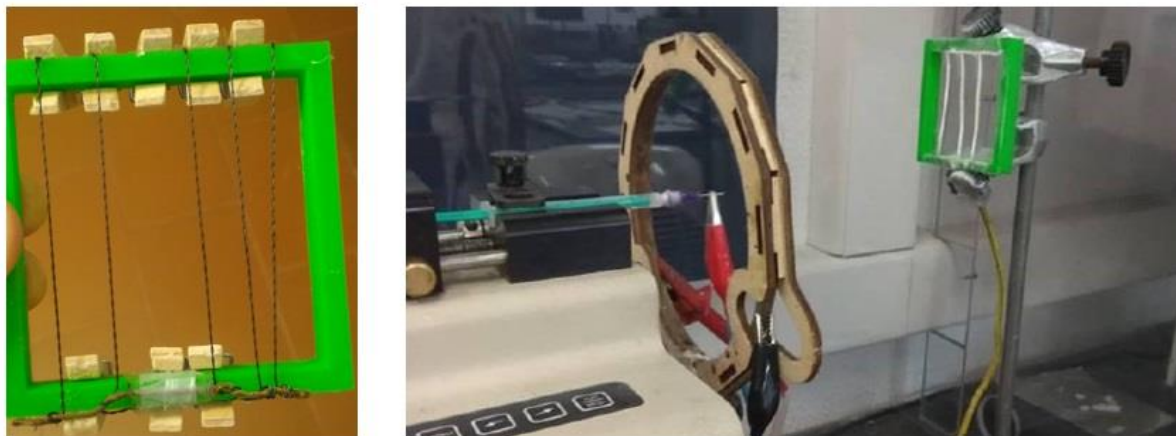
Figure B. 1 - left: Photo of the frame used to support the carbon threads during electrospinning. Right: photo of a similar electrospinning setup from [42].
