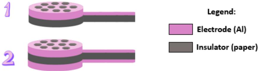
Figure 3.3 - Schematics of the generator configurations used: (1) One electrode; (2) Two electrodes.
