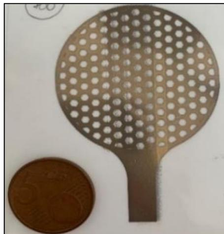
Figure B.1 - Photographs of the generators made by inkjet printing. A 5-cent coin for scale purposes (21.25mm in diameter).
