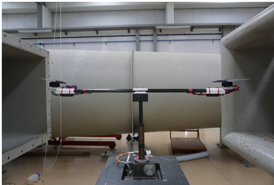
Figure 6.9: Boom with VTOL system to be tested in the wind tunnel.
