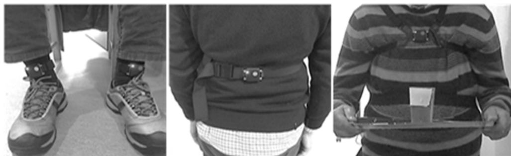
Figure 1. Placement of the Opal sensors and tray with a glass of water.
