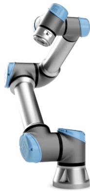
Figure 5.2: Universal Robots UR5e collaborative robotic arm.
