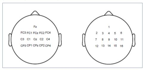
Fig. 5 Layout of the used 16 EEG channels cap.
