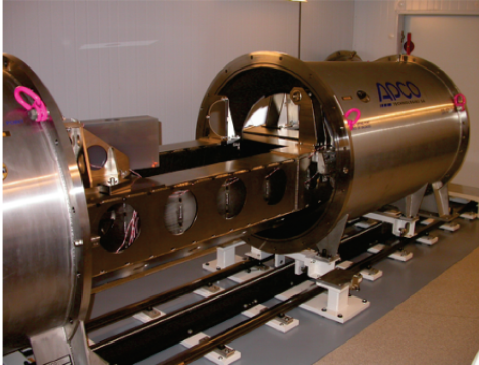
Figure 2.3: The HARPS spectrograph inside the air-conditioned room at La Silla just before being closed and evacuated (from Mayor et al. 2003).
