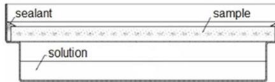
Figure 60. Scheme of the assembly for the wet-cup measurements (Ramos 2007)
