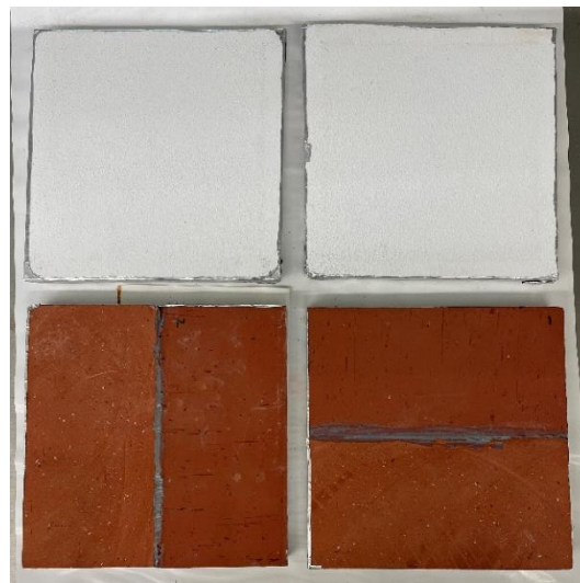
Figure 59. Specimens of brick and insulating render system for the water vapour permeability test.
