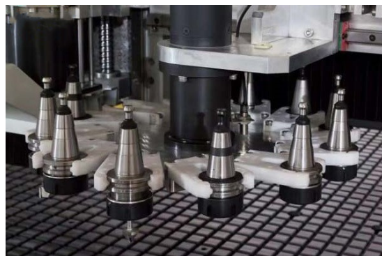
(b) IEHK ATC 1325 CNC Router with Servo automatic tool changer.
