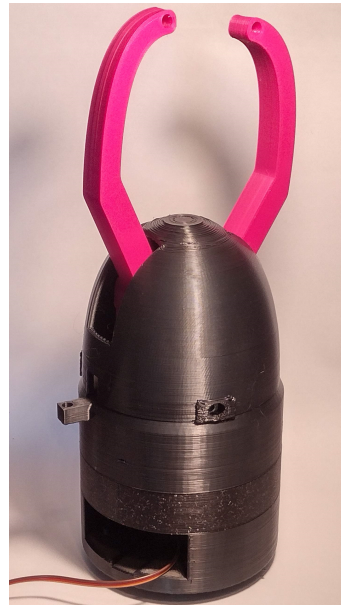
Figure 4.8: Example of an assembled tool changer with a 2 finger gripper protection housing.
