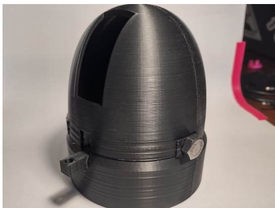
(a) Example Protection Housing for a 2 finger gripper configuration mounted on a standard Tool Side Interface.
