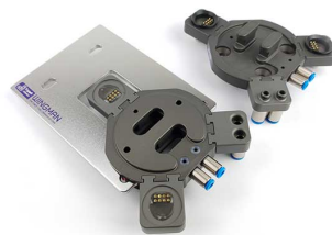
(b) TripleA Robotics: WING-MAN - Automatic and Manual Tool Changer.
