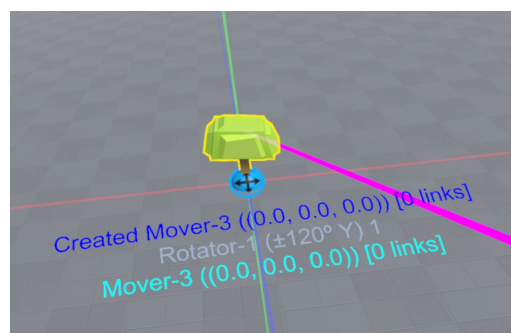
Figure 4.12: Live feed. In the first panel the feed shows all three components, just after a user wrapped a Rotator object (hovered) with a Mover object and entered edit mode.
