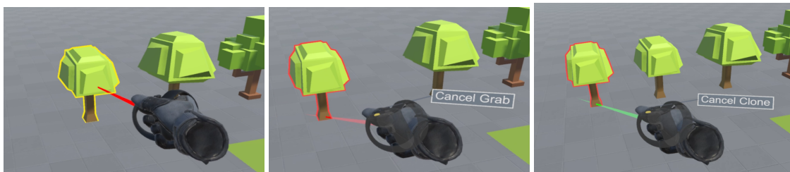
Figure 4.1: Hovering over a tree object. In the middle panel the user is in grab mode and moves the tree. In the right panel the user is in clone mode instead, and the cloned tree is immediately grabbed.
