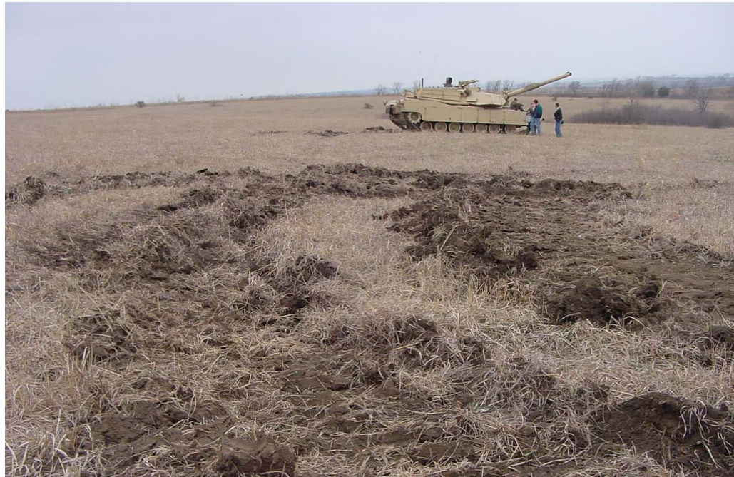
Figure 1-2 Soil disturbance caused by a tank on a single pass (St.Clair, 2007)
