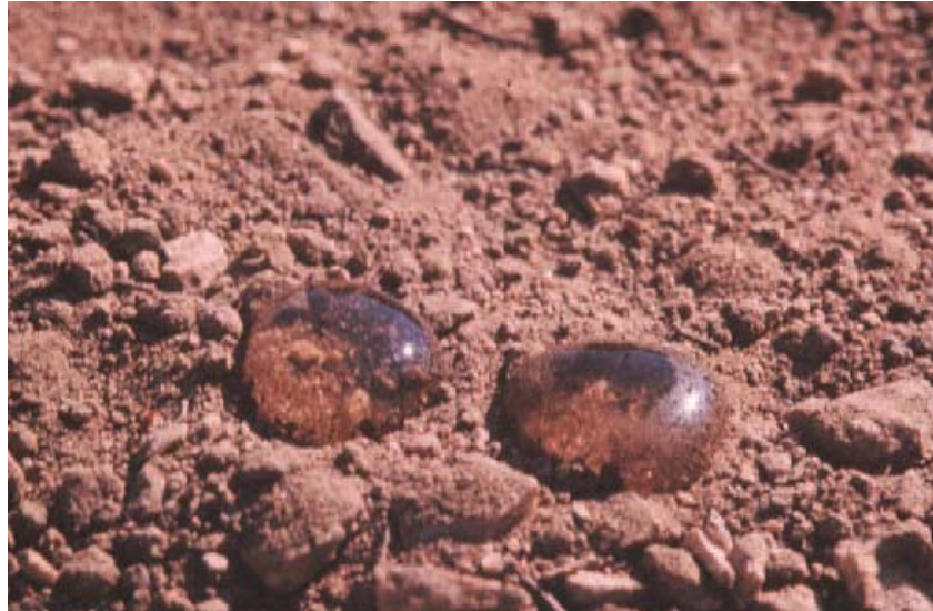
Figure 1-6 Beading effect of water droplets on a water repellent soil (Neary et al., 2005).
