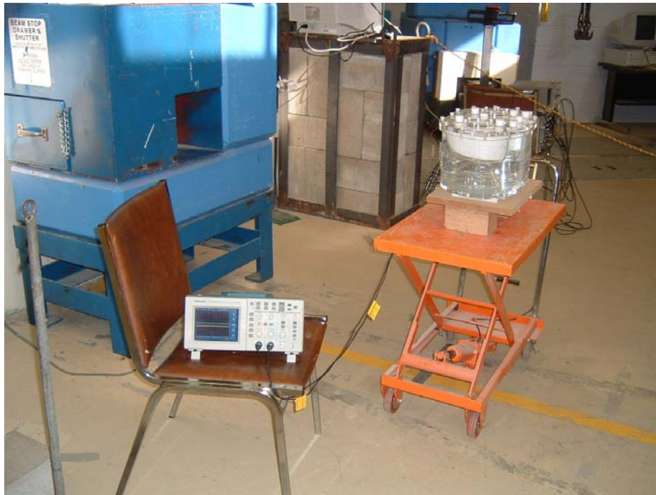
Figure 4.11. Semiconductor-Based Neutron Dosimeter Experiment in the Beam Port.
