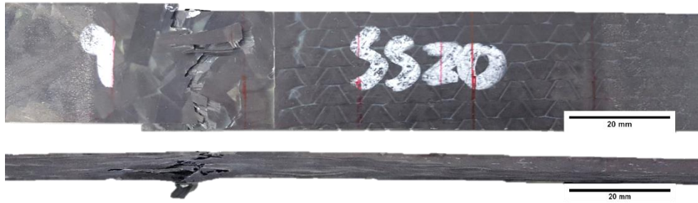
Figure 13. Failure of a tensile specimen with a step size of 20h (6mm), where failure occurs within the DFC region away from the joint
