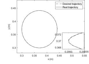
Figure 9 3D position behavior of UR5 using the proposed controller in x-y plane
