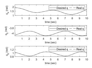
Figure 6 trajectory tracking behaviour of the robot using the proposed approach for the last three joints
