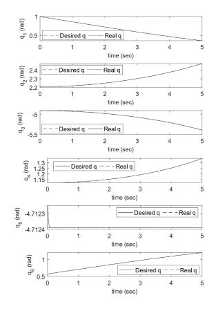
Figure 2 Joint angle behavior of UR5 using the proposed control approach
