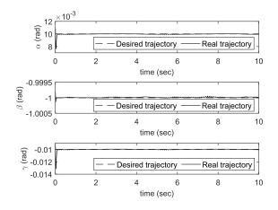
Figure 8 3D orientation behavior of UR5 in the presence of the proposed controller
