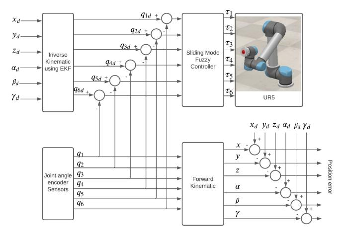
Figure 1 Overall block diagram of the proposed controller
