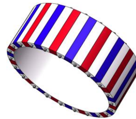
Fig. 13. 3D structure of the outer rotor
