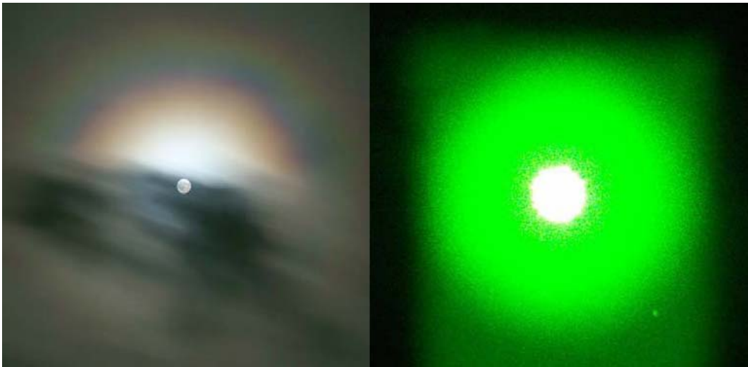
Figure 3.2 The picture 5 on the left shows a lunar corona caused by the small clouds droplets. The right picture shows a halo caused by scattering from a suspension of 9.6 \mu\text{m} polystyrene particles in water; the white circle in the center is due to the saturation of the CCD camera.
