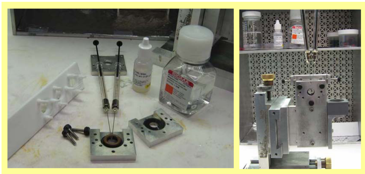
Figure 5.7 The scattering cell (left) and the sample holder (right) are shown. The solutions are injected into the cell through two holes inserted in the O-ring. The metal sample holder has a hole centered on the quartz windows. The sample is mounted onto the translation stage for SALS measurements
