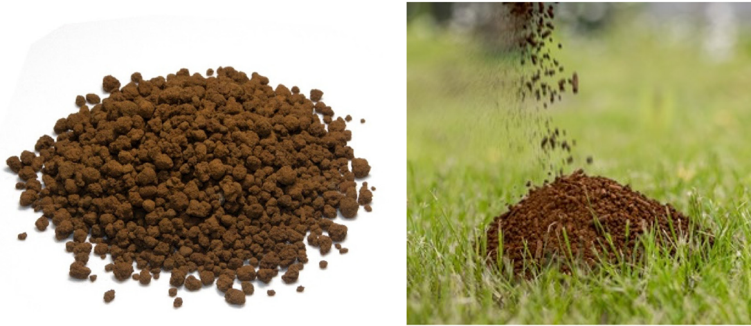
Figure 12.6 Iron oxide pellets produced from iron-rich ground water sludge (photo credits: Olaf van der Kolk, AquaMinerals).
