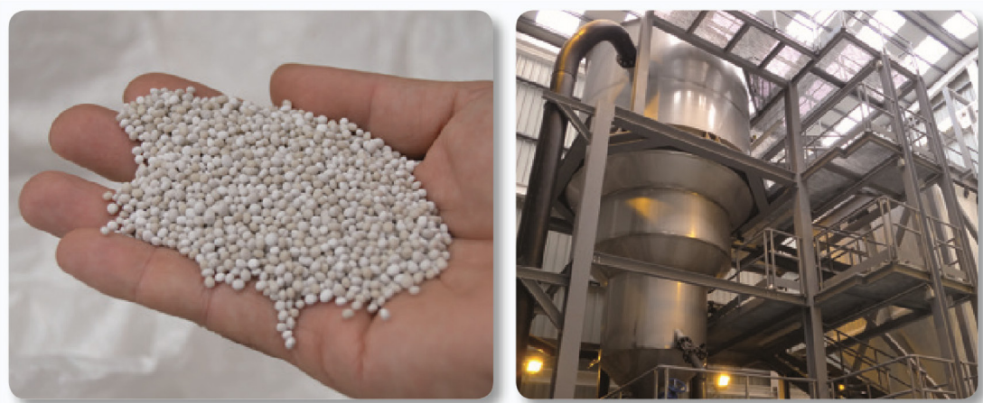
Figure 10.17 Ostara® struvite granules commercialized as Crystal Green® Ostara pearls (left) and Pearl® Technology reactor (right).
