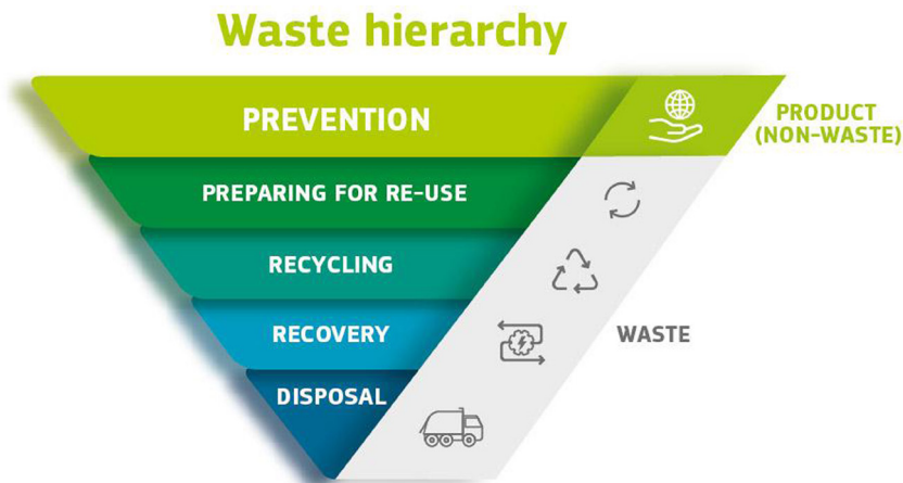
Figure 13.1 Waste hierarchy as stipulated in the waste framework directive (source: European Commission, 2008 ).
