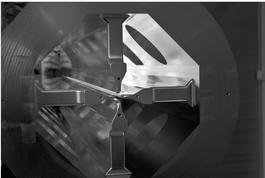
FIGURE 3.52 Four-vane RFQ for Linac4 at CERN; image courtesy of CERN.
