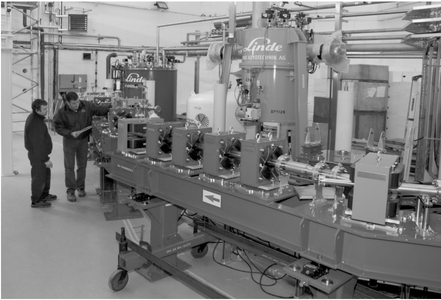
FIGURE 1.2 Part of the ALICE energy-recovery linac electron beam transport system, previously installed at Daresbury Laboratory. Individual beamline magnets are typically mounted onto a girder (usually steel), adjusted so that their magnet centres are aligned and then fixed (with position accuracy of some tens of \mu\text{m} ); the girder may then be lifted into its operating position without significant relative movement of the magnets, and they may be adjusted together for efficiency. A typical alignment accuracy from girder to girder of a few tens of \mu\text{m} is also commonly achieved. ©STFC
