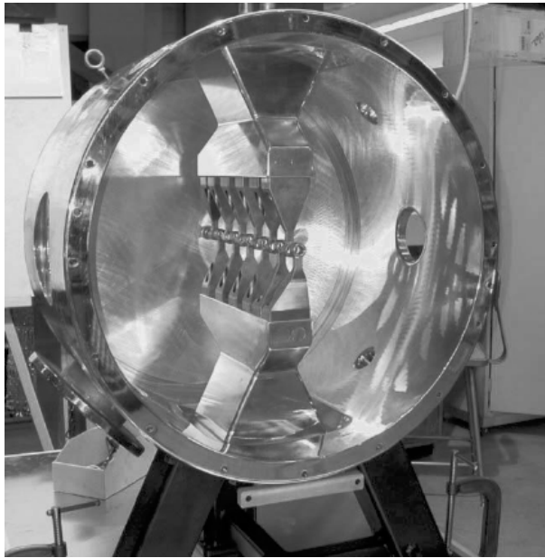
FIGURE 3.51 IH (interdigital H-mode) resonator for ISAC radioactive ion beam facility at TRIUMF; [62]
