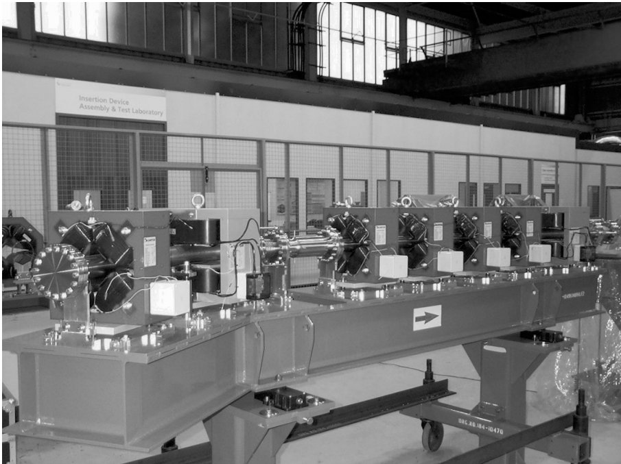
FIGURE 5.7 A beamline section for a so-called transfer line between two accelerators, showing an arrangement of focusing and defocusing quadrupoles (with four poles), dipoles (with two poles), and intervening drift spaces, mounted on a common supporting girder. © STFC
