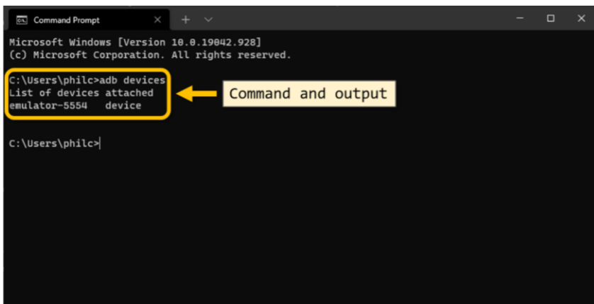
Fig. 8.17: ADB Walkthrough - “adb devices” Command
