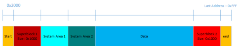
Fig. 4.1: Layout of a QNX6 filesystem volume
