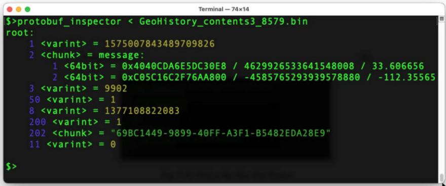
Fig. 9.32: Protobuf-Inspector converted Hex values. Lat and Long?
