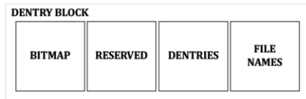
Fig. 3.14: F2FS Dentry Block Structure
