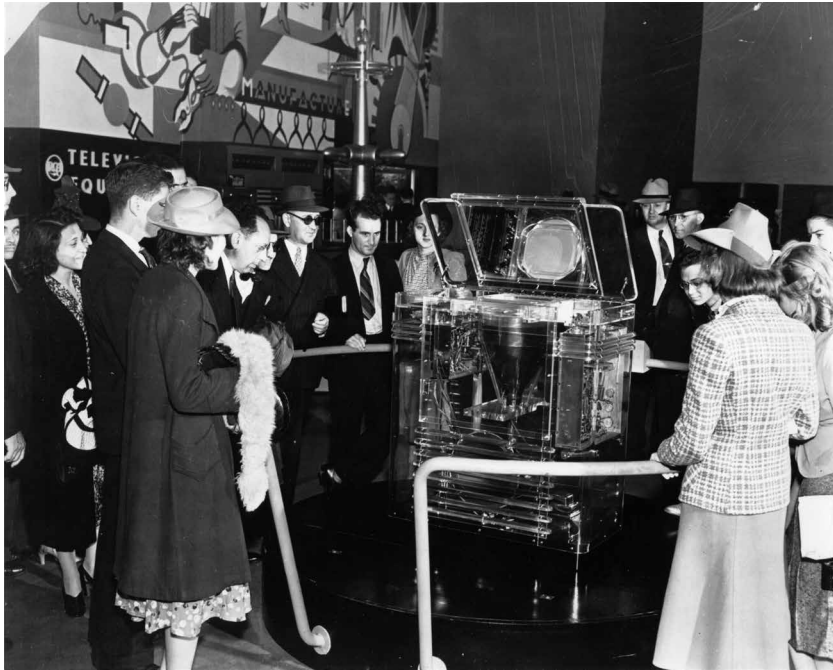
Figure 5.20. RCA's so-called 'Phantom Receiver', a TRK-12 model television with a plastic cabinet. Source: RCA News and Information Department photographs (Accession 2464.68), Box AVD3, Folder 10, Hagley Library and Archives.
