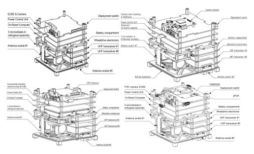
**Figure 4.1:** Evolution of the payloads on BEESAT. Top left: BEESAT-1 (CAD-model created by Sebastian Trowitzsch, image credit: Diego Garcia). Top right: BEESAT-2 (CAD-model adapted by Sebastian Trowitzsch, image credit: Sebastian Trowitzsch). Bottom left: BEESAT-4 (CAD-model adapted by the author). Bottom right: (CAD-model adapted by Sebastian Grau, image credit: Diego Garcia)
