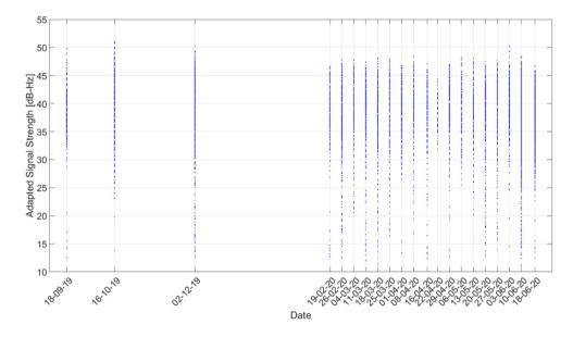
Figure 7.16: Accumulated signal strengths of GNSS satellites during the mission
