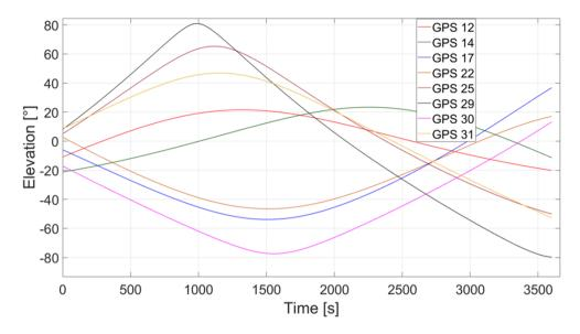
Figure 6.5: Elevation of GPS satellites over the antenna of BEESAT-4
