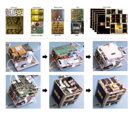
Figure 5.1: Integration process of BEESAT-4
