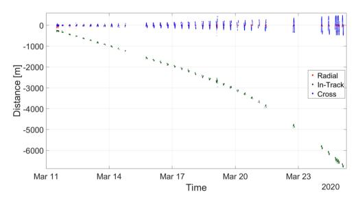
Figure F.23: Orbit propagation of two weeks from 2020-03-10, based on one orbit of GNSS data
