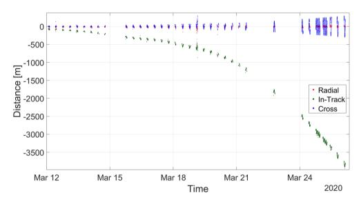
Figure F.21: Orbit propagation of two weeks from 2020-03-10, based on 10h of GNSS data
