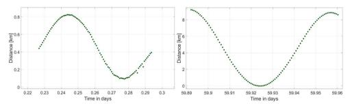
Figure 7.7: In-track amplitude change over two months of the "best" TLE
