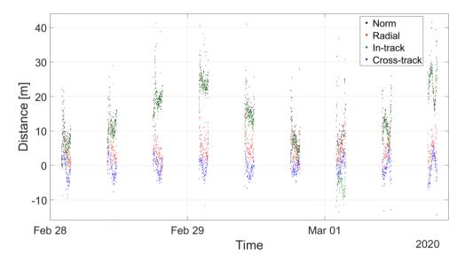
Figure F.1: Residuals for a three day GNSS data set from 2020-02-28
