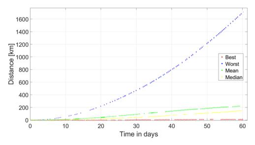
**Figure 7.14:** Differences from GNSS to SGP4 for all three directions for the "worst" TLE with a modified B\* value
