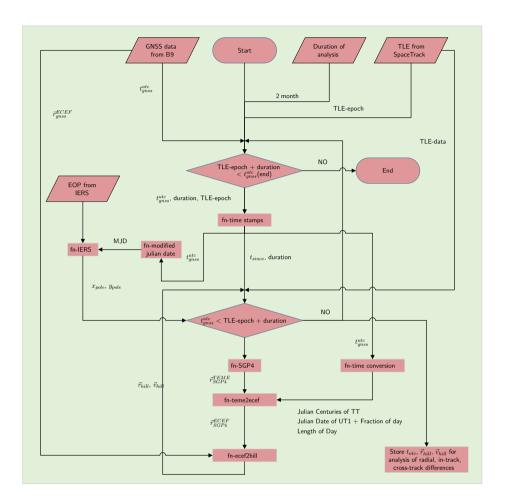
Figure 7.4: Flowchart of calculation of distances betweens GNSS and TLE ephemerides
