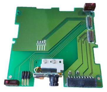
Figure 4.9: EGSE and camera board of BEESAT-1
