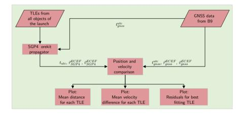
Figure 7.1: Flowchart of object identification of BEESAT-9
