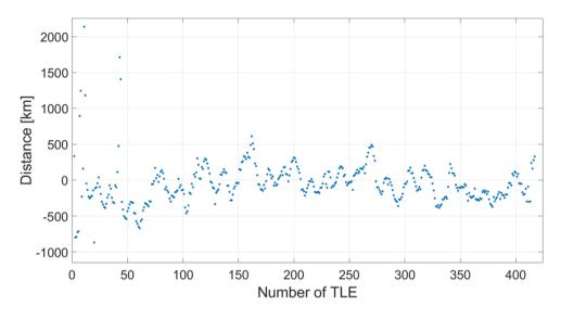
Figure 7.9: Maximum in-track difference after two months for all TLEs
