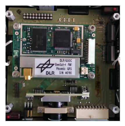
Figure 4.11: PDH with GPS receiver and camera
