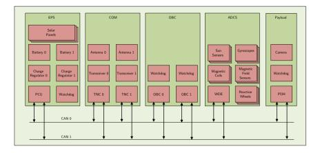
Figure 4.2: System overview of the subsystems of BEESAT-1 (adapted from [132])
