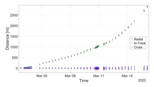
Figure F.11: Orbit propagation of two weeks from 2020-02-29, based on two days of GNSS data
