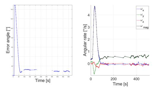
**Figure 6.4:** Control error angle and angular rates of BEESAT-4 during zenith pointing [170]
