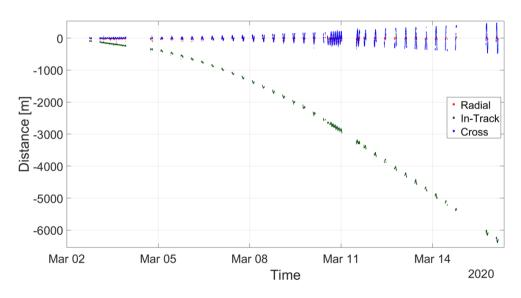
Figure F.15: Orbit propagation of two weeks from 2020-03-01, based on one orbit of GNSS data
