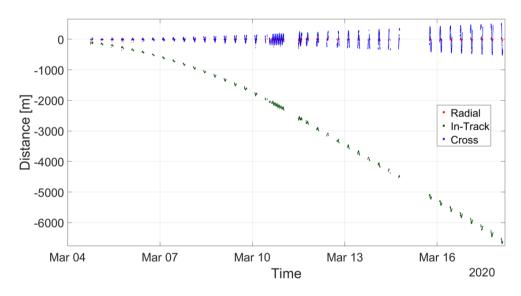
Figure F.19: Orbit propagation of two weeks from 2020-03-03, based on one orbit of GNSS data
