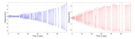
Figure 7.8: Cross-track (left) and radial (right) difference development over two months
