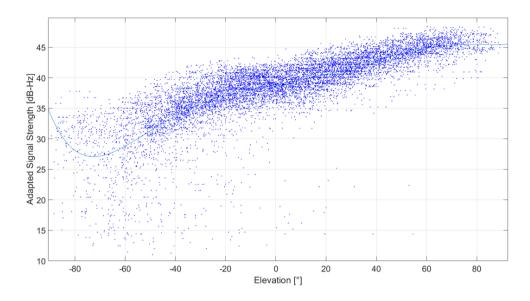
Figure 7.17: Carrier Signal-to-Noise Ratio of tracked GNSS satellites depending on elevation
