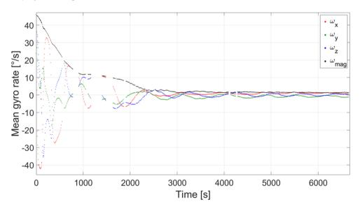
Figure 6.3: Angular rates during Blind Damping Mode (adapted from [188])
