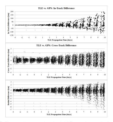
**Figure 2.3:** The in-track, cross-track, and radial differences between the AeroCube-4B GPS fixes and SGP-4 propagated TLE [87] (*Courtesy of and reprinted by permission of The Aerospace Corporation.*)
