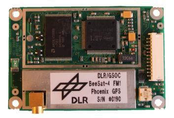
Figure 2.4: Flight model of the Phoenix GPS receiver for BEESAT-4
