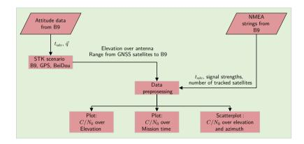
Figure 7.15: Flowchart of calculation of signal strengths over elevation
