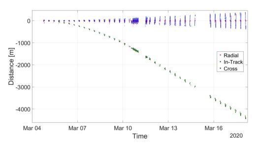
Figure F.17: Orbit propagation of two weeks from 2020-03-01, based on 20h of GNSS data
