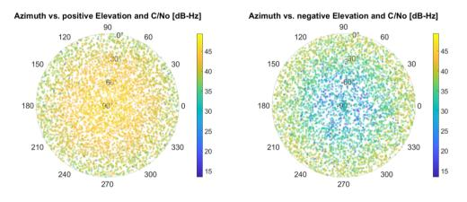
Figure 7.18: Carrier Signal-to-Noise Ratio over elevation and azimuth
