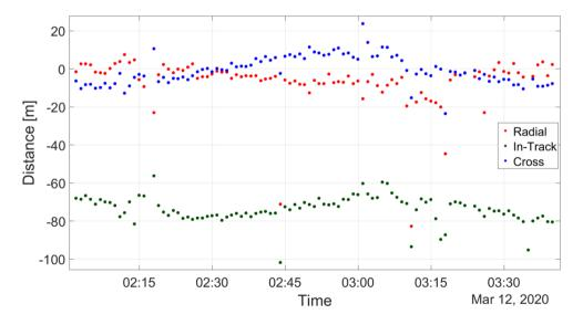
Figure 7.21: In-track, cross-track and radial difference 24h after last GNSS data input
