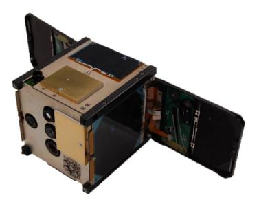
**Figure 2.1:** Flight model of AeroCube-4 [103] (*Courtesy of and reprinted by permission of The Aerospace Corporation.*)
