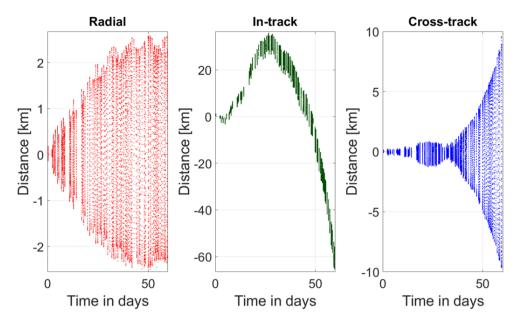
**Figure 7.13:** Differences from GNSS to SGP4 for all three directions for the "worst" TLE with a modified B\* value
