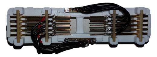
Figure 5.7: Adapter for the GNSS200 (built by Sebastian Grau)
