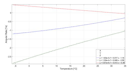
Figure 5.4: Temperature dependency of the offset of gyroscope MAX21000
