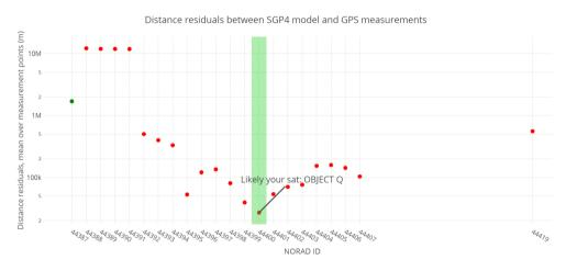
Figure 7.2: Object identification on 2019-07-07, GNSS data compared to TLEs (image credit: Clément Jonglez)
