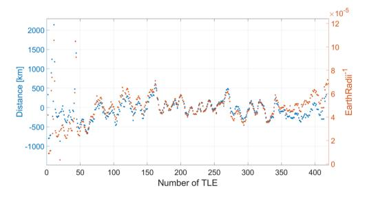
Figure 7.11: Correlation between in-track difference and B\*
