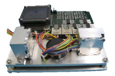
Figure 4.7: Reaction wheel system with WDE [132]
