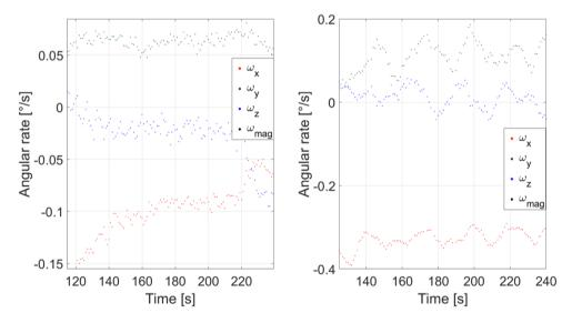
**Figure 6.9:** Comparison of angular rate between the sensors, left side: BMG250, right side: MAX21000
