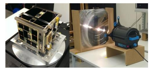
Figure 5.3: Setup for the calibration of sun sensors on BEESAT-4
