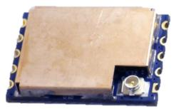
Figure 2.5: FM of GNSS200 for BEESAT-9 (image credit: Hyperion Technologies [53])
