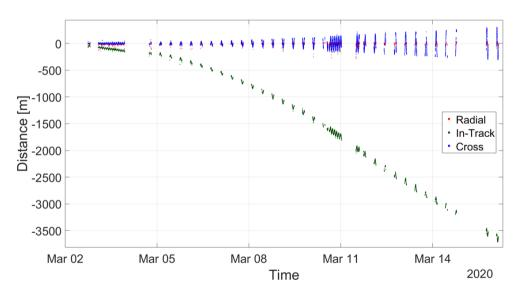
Figure F.9: Orbit propagation of two weeks from 2020-02-28, based on three days of GNSS data
