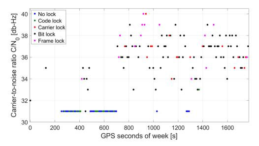
Figure 5.2: Lock status in relation to signal strengths of the Phoenix receiver
