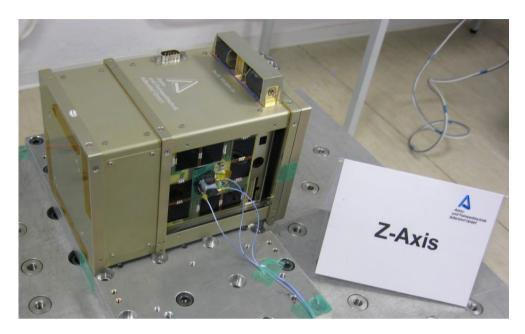
Figure 5.5: BEESAT-4 on the shaker in an SPL
