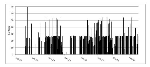
**Figure 2.2:** GPS fixes of AeroCube-4B and Aerocube 4C for the first eight months in orbit [87] (*Courtesy of and reprinted by permission of The Aerospace Corporation.*)
