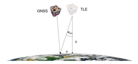
Figure 7.5: Calculation of limit for a TLE update
