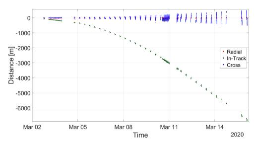
Figure F.13: Orbit propagation of two weeks from 2020-03-01, based on three orbits of GNSS data
