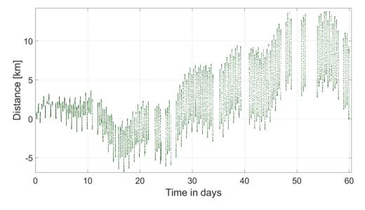
to 1 km for BEESAT-9. In Figure 7.6, the in-track difference is displayed for a duration of two months including 148 navigation experiments.
