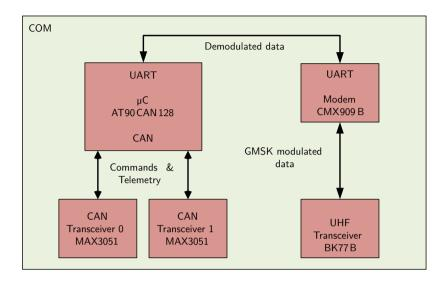
Figure 4.3: Schematic configuration of the communication system (adapted from [132])
