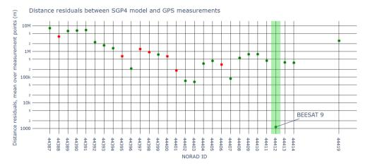
**Figure 7.3:** Object identification on 2019-07-17, GNSS data compared to TLEs (image credit: Clément Jonglez, rerun by the author)
