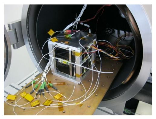
Figure 5.6: BEESAT-4 in a thermal vacuum chamber
