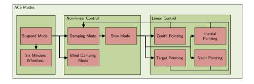
Figure 4.8: Modes of the ADCS (adapted from [132])
