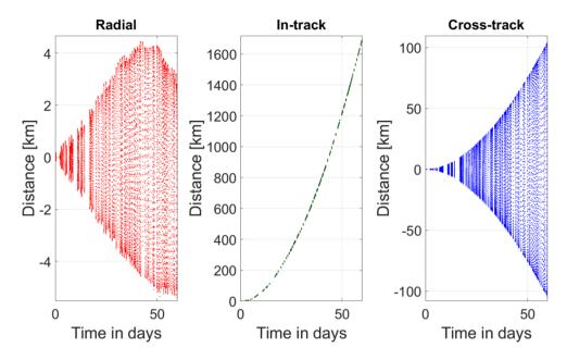
Figure 7.12: Differences from GNSS to SGP4 for all three directions for the "worst" TLE
