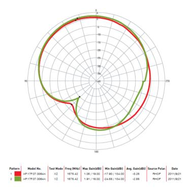
Figure 4.14: Radiation pattern of GNSS antenna of BEESAT-9 [163]
