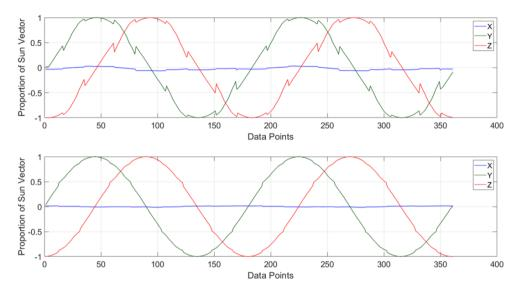
**Figure 5.8:** Sun sensors of BEESAT-9 before (top) and after (bottom) calibration (adapted from [182])
