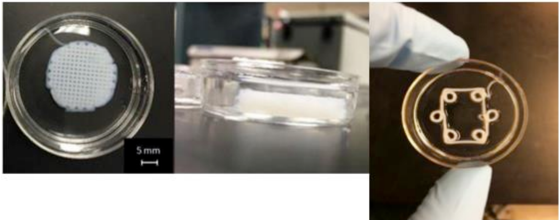
Figure 8.2. Collagen scaffolds printed from the custom 3D printer (A) top view of a 20 mm X 6.3 mm 3D printed collagen cylinder scaffold (B) side view of a 20 mm X 6.3 mm 3D printed collagen cylinder scaffold (C) 4 mm X 2.4 mm 3D printed cylinder scaffolds used for experimentation.
