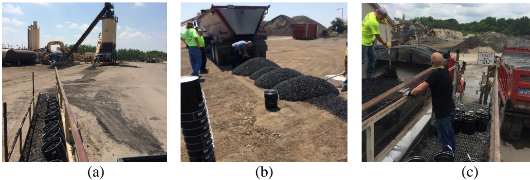
Figure 3-1. Sampling plant produced mixtures from different asphalt plants. a) Mix 1836, Wm Ch; b) Mix 1845, Curran, and; c) Mix 1807, Geneva
