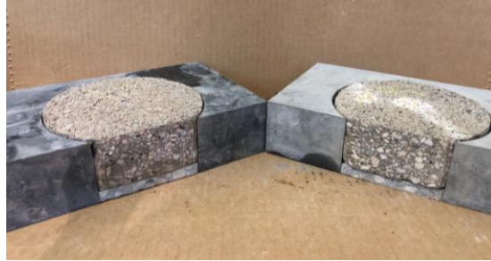
Figure 2-14. Hamburg samples with 12mm PCC shims placed below asphalt specimens
