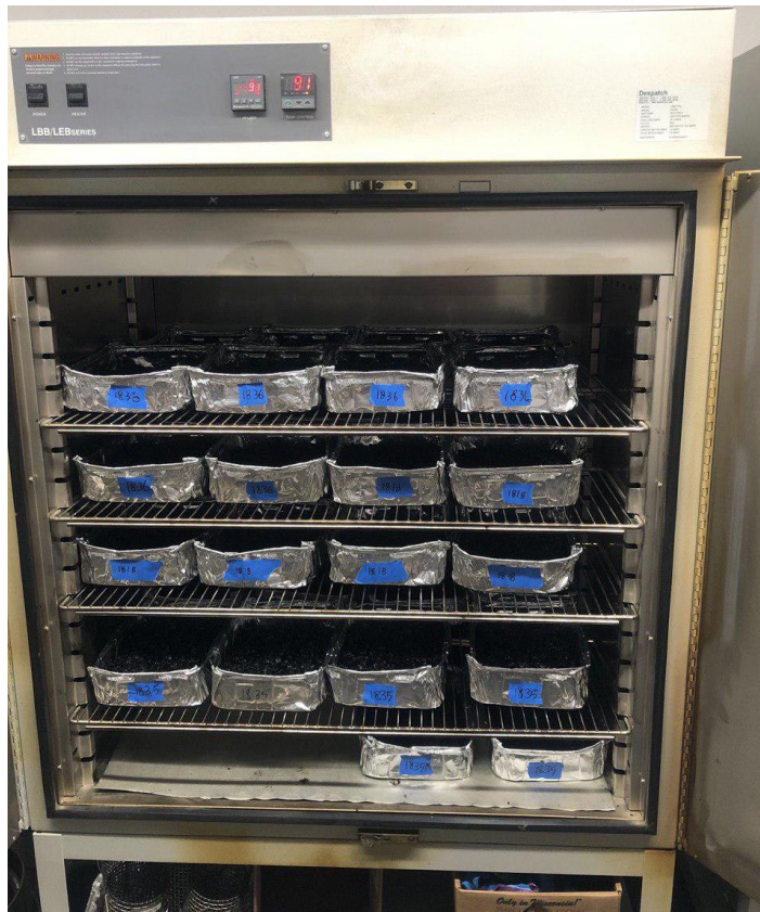
Figure 3-23. Aging the Tollway 2018 plant produced mixtures in oven at 95 °C for 6 days
