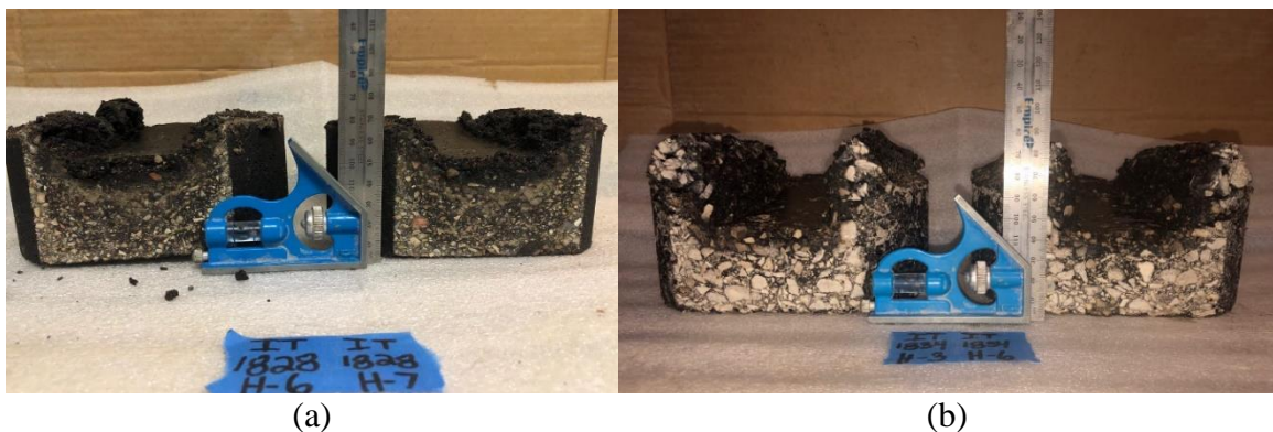
Figure 3-14. Tested samples after 20K pass at 50 °C. a) 1828 mix, b) 1834 mix
