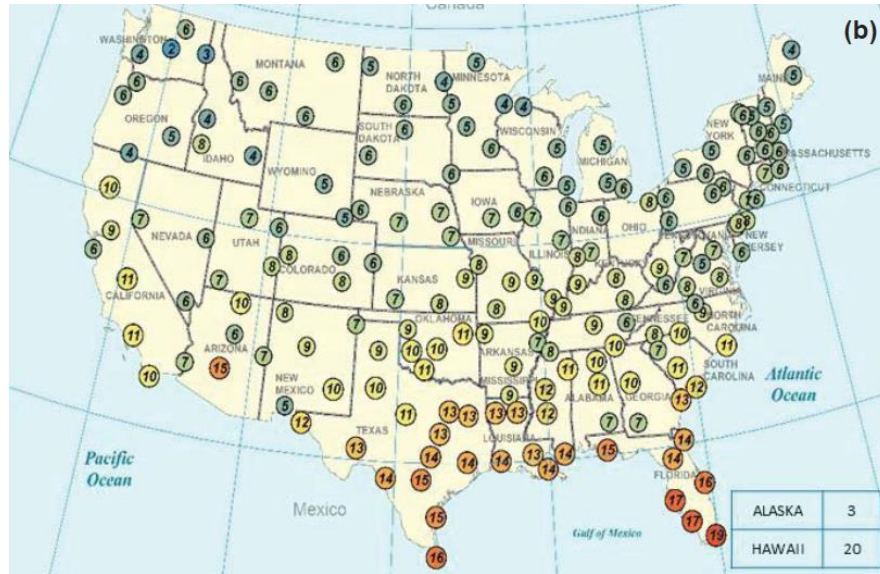
Figure 3-22. Required oven aging durations at 95°C to match level of field aging 6 mm below pavement surface for 8 years of field aging (Kim et al., 2018)
