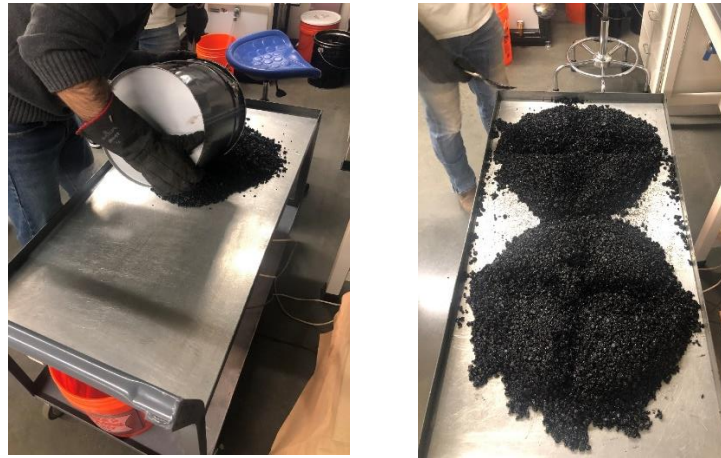
Figure 3-5. Splitting the bucket of mixture as per AASHTO R47
