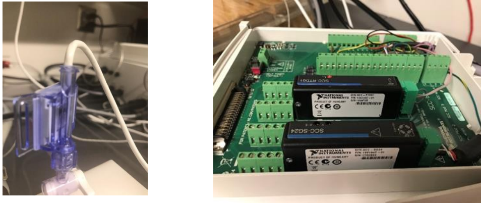
Figure 4-10. a-Pressure transducer, b- picture of the SCC-SG24 Wheatstone bridge and amplifier.
