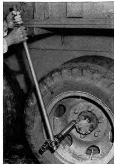
Made For Tough Nuts. It's a geared nut tightener (and loosener) made for heavy-duty use. The device uses Shelby Seamless Mechanical Tubing for maximum strength. USS Shelby Tubing is actually pierced from a solid billet of fine steel. The tubing is hot worked and forged in the process, and it contains no welds.
