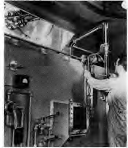
Laboratory workers handling "hot" atoms work behind barricades. Here an operator, using a remote-control instrument, watches in a mirror as he siphons a radioisotope solution into a bottle.
