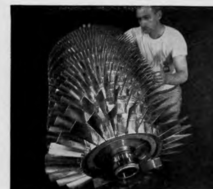
Design of a multi-stage, axial-flow compressor involves some of the most complex problems in the entire field of aerodynamics. The work of aerodynamicists ultimately determines those aspects of blade and total rotor design that are crucial.
