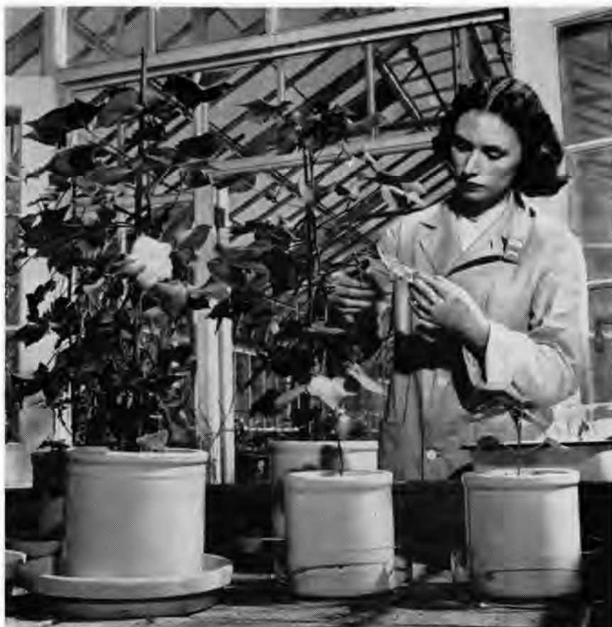
Agricultural researchers "tag" fertilizers with radioactive phosphorus. Then by exposing the leaves of plants to film, they can tell how well the nutrient has been distributed through the plant and thus how effective is the fertilizer.
