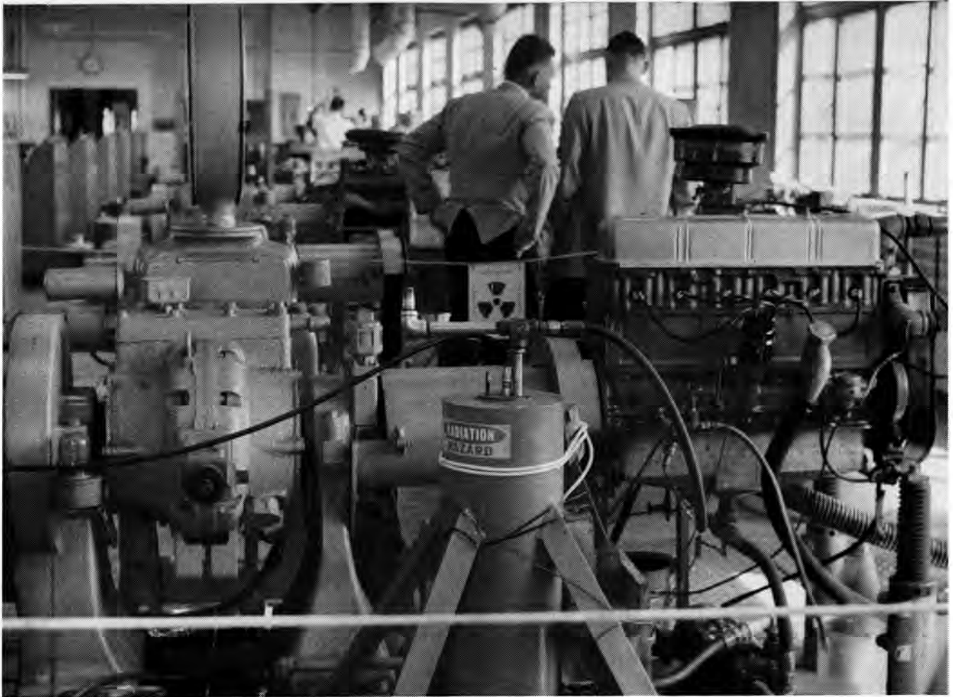
Modern and advanced engines log up hundreds of test hours daily in Standard's automotive laboratory at Whiting. Radioactive carbon traces deposits in the guarded engine (foreground).
