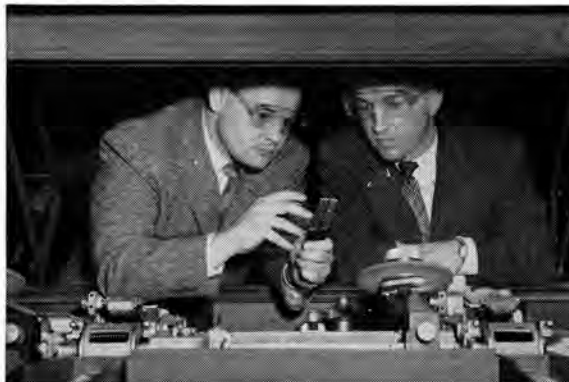
Examining the plastic molded "comb" components of the wire spring relay Dick recalls his early work when he was involved in working-up forming and coining tools for the pilot model of the automation line for fabrication of wire spring sub-assemblies for relays. At present he is associated with the expansion of these automation lines at the Montgomery Plant.
