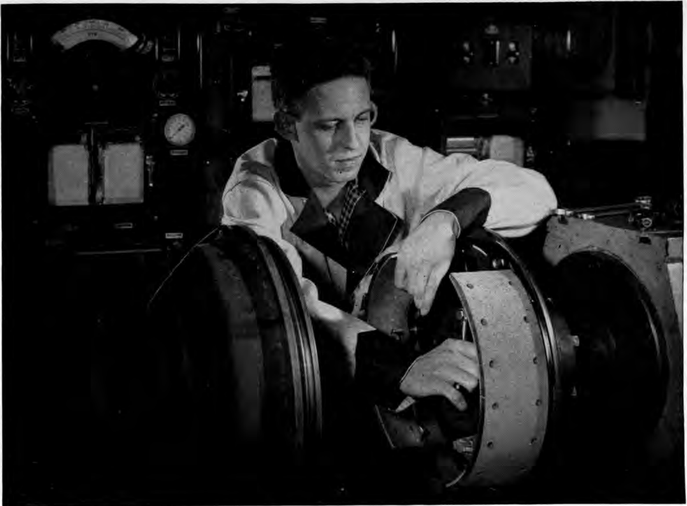
Installing a hydraulic brake assembly on the dynamometer in the Wagner Research Laboratory
