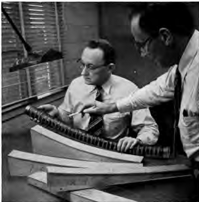
One type of guide, designed to be flexible, is bent on wooden forms to study effect of curvature on transmission. Left is A. C. Beck, Radio Research Engineer, E.E., Rensselaer Polytechnic Institute. Right is A. P. King, Radio Research Engineer, A.B. in Physics and Engineering, California Institute of Technology.
