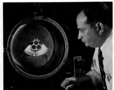
'NEW LOOK' AT 'SHELL' OF NUCLEAR REACTOR —These patterns of light show the stresses inside the "shell" of a power-producing nuclear reactor.
