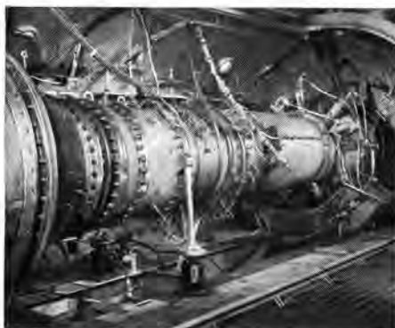
Mounting an afterburner in a special high-altitude test chamber in P&WA's Willgoos Turbine Laboratory permits study of a variety of combustion problems which may be encountered during later development stages.
