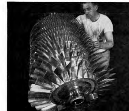
Design of a multi-stage, axial-flow compressor involves some of the most complex problems in the entire field of aerodynamics. The work of aerodynamicists ultimately determines those aspects of blade and total rotor design that are crucial.
