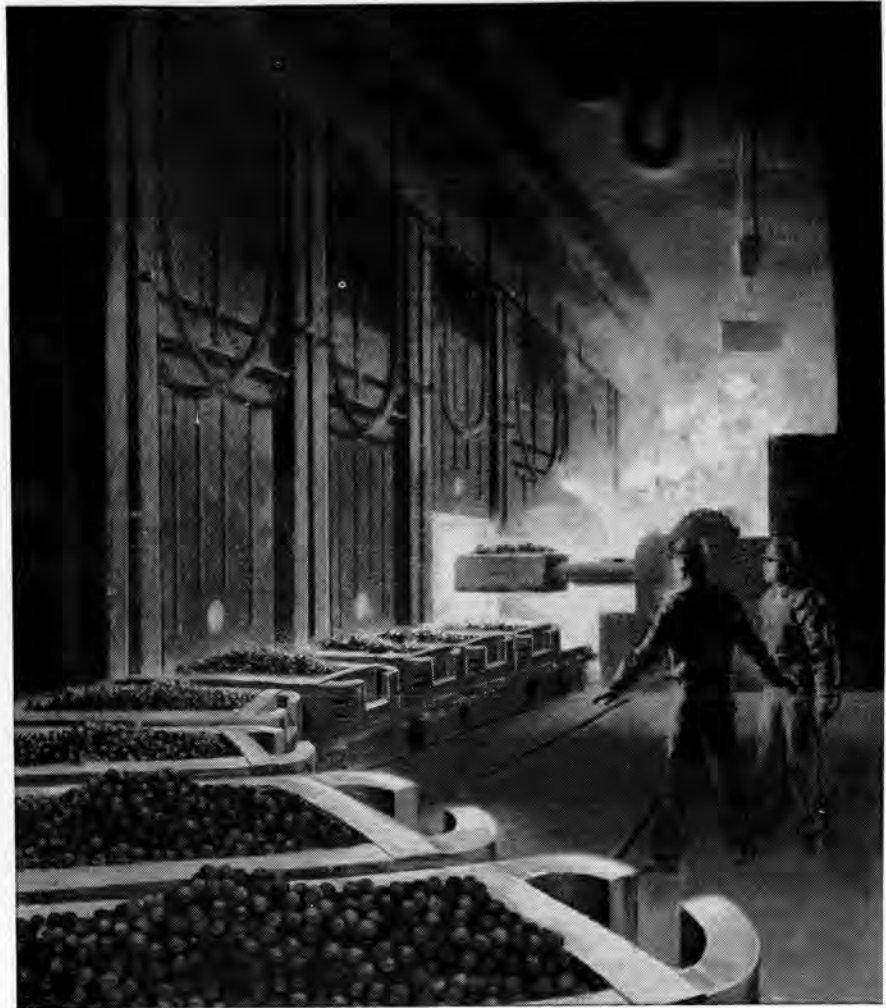
Now this high-grade iron ore—product of Inco research—goes to steel mills. Here you see it being fed into open hearth furnaces.
