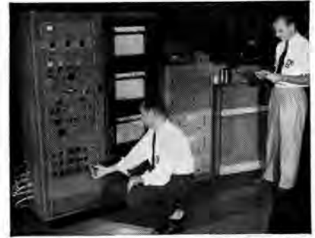
The "Plottomat", designed by P & W A instrumentation engineers, records pressure, temperature and air flow direction. It is typical of an expanding program in automatic data recording and handling.
