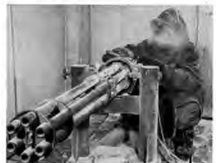
FIRE GOD ON ICE —Here, G.E.'s Vulcan defies arctic cold and performs satisfactorily at temperatures down to 70 below zero. Tested under arctic and high altitude conditions the gun showed its remarkable versatility.
