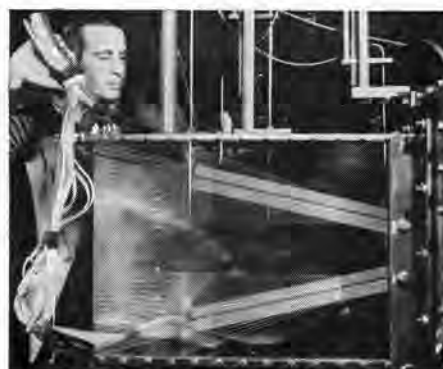
Pratt & Whitney Aircraft engineer manipulates probe in exit of two-dimensional research diffuser. Diffuser design for advanced power plants is one of many air flow problems that exist in combustion work.
