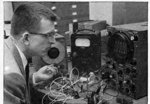
Pratt & Whitney Aircraft engineer checks a bread board model for a subminiature, encapsulated amplifier built with transistors.
