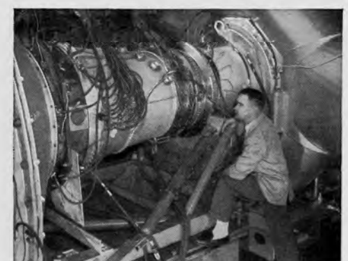
Mounting a compressor in a special high-altitude test chamber in P & W A's Willgoos Turbine Laboratory permits study of a variety of performance problems that may be encountered during later development stages.
