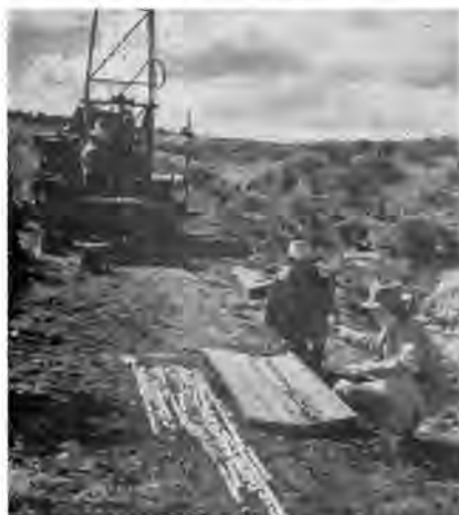
Cores recovered by an exploratory diamond-drilling operation are being examined by a geologist to see if there are any traces of uranium ore.
