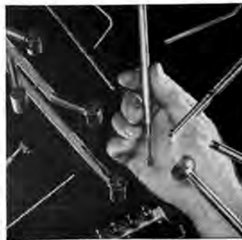
Special-purpose probes designed and developed by P & W A engineers for sensing temperature, pressure and air flow direction at critical internal locations.
