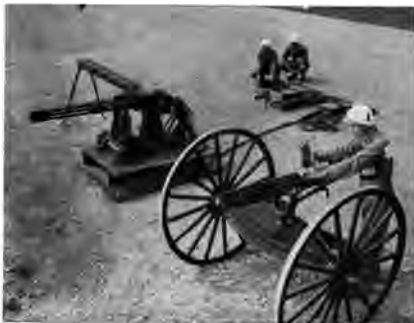
FIRE GOD —New "Vulcan" gun (left), named after Roman God of Fire, fast firing 20 millimeter aircraft cannon, developed and manufactured by General Electric under Army Ordnance direction for U.S. Air Force, is shown with its famous 19th-century predecessor, the Gatling Gun.
