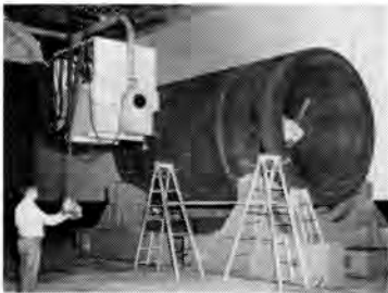
Radiographs of the reactor vessel welds were made with a 15,000,000-volt betatron. Every bit of the special steel, every weld had to be proved sound and flawless.
