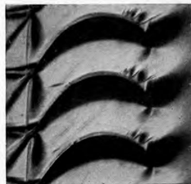
Schlieren photographs, above and left, illustrate different phases of airflow investigation. Development of inlets, compressors and turbines requires many such studies in cascade test rigs, subsonic or supersonic wind tunnels.
