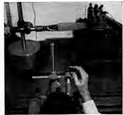
P & W A engineer uses air jet to vibrate compressor blade at its natural frequency, measuring amplitude with a cathetometer. Similar fatigue tests use electromagnetic excitation.
