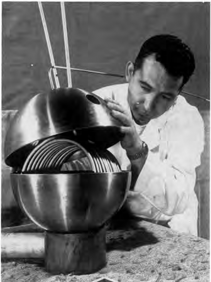
Physicist checks core for nuclear research reactor built for the Armour Research Foundation of Chicago. Atomic fission, the "splitting" of atoms which produces radioactivity and neutrons, takes place in this heavy stainless steel core.
