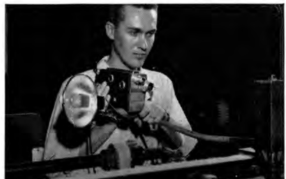
A motion picture camera, adapted for single shots with "strobe" flash, snaps thousands of readings on a roll of film.
