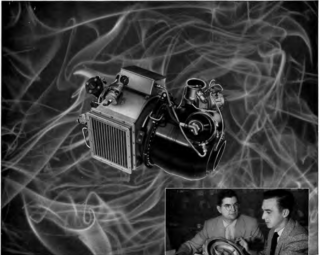
AiResearch two stage lightweight gas turbine compressor provides pneumatic power for aircraft main engine starting and serves as auxiliary power source for a variety of ground and in-flight services.
