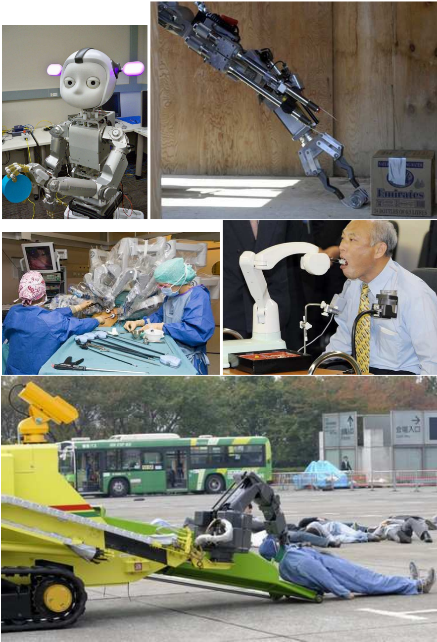
Figure 16.2: Various cyborgs, from top to bottom and left to right: a cyborg by PlasticPals, named Simon, based on imitation learning; the two following robots, based on human (remote) pilots, are maybe less elegant but more efficient: a cyborg setting up a small bomb for destroying a dangerous packet; a medical robot for surgery. The next robot is here for helping disabled people; the last robot picks up irradiated bodies (4 last images from botson.com).
