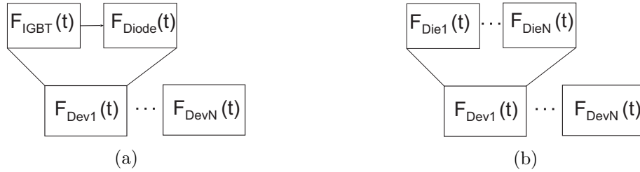
Figure 3.14: Series-connected reliability modeling, whereby the failure of a single component means system interruption, for the procedures: (a) System-Level Design for Reliability (b) Die-Level Design for Reliability.
