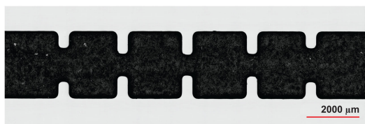
FIGURE 7. Laser-microscope view of a single laser-induced filter throughout the structured-glass wafer shown in Fig. 6.
