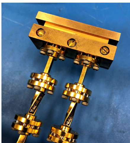
FIGURE 10. Assembled prototype and split-block interface attached to the test-bed.
