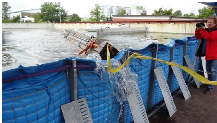
Figure 1.2: Exemplary experimental impact analysis for flood barrier flexible structures in TU Hamburg-Harburg (Wibbeler 2016) [2]
