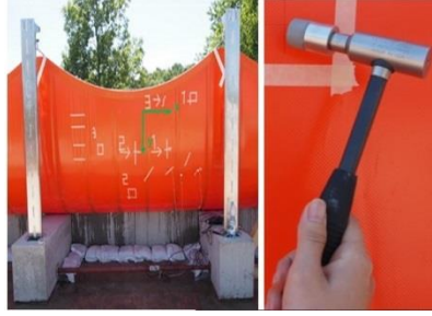
Figure 2.1: The textile flexible membrane prototype and the impact hammer
