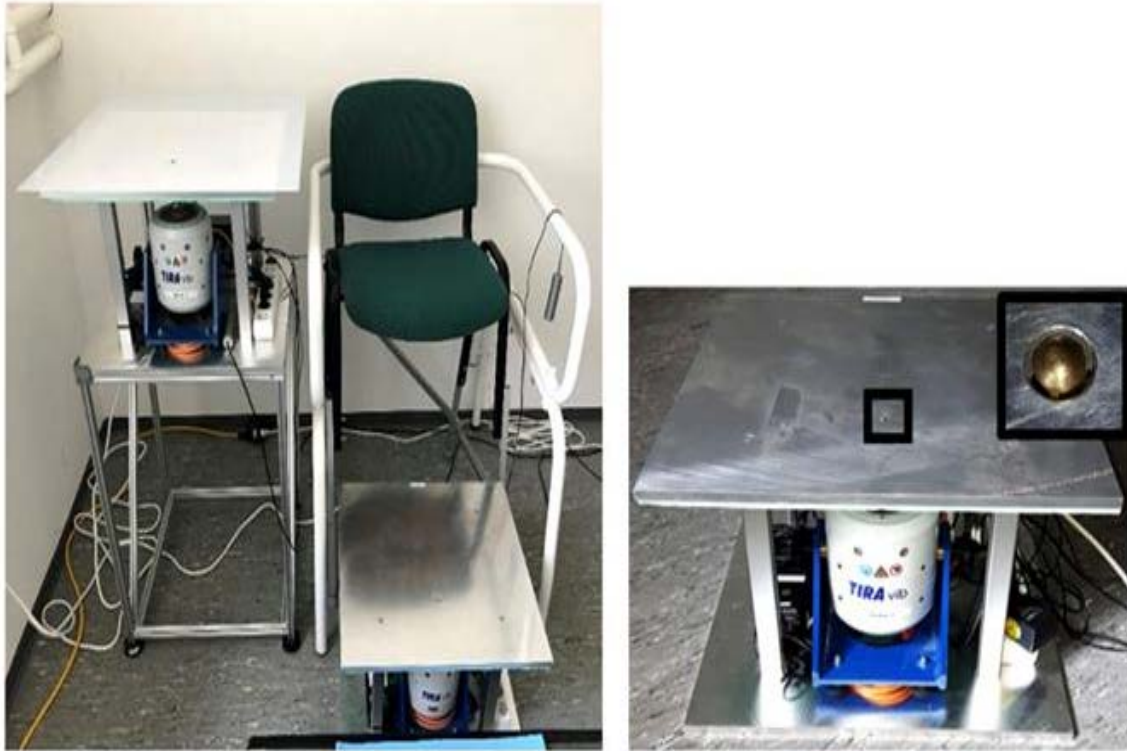
Fig. 7 Left: Vibration perception threshold set-up for measuring hand and foot sensitivity. Right: Platform with tip of vibrating probe (black squares).
