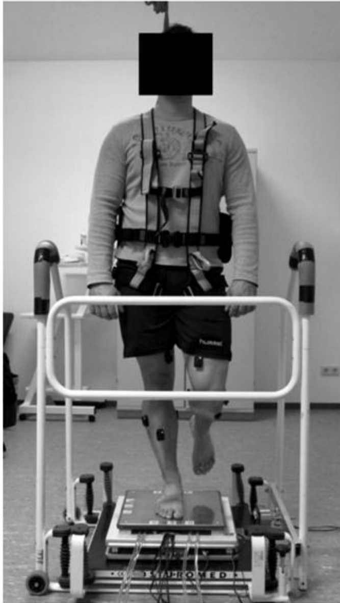
Fig. 1 Picture of the apparatus used. Subjects stood with their dominant leg on top of the thermal plate which was mounted on top of the force platform. The force platform was then placed on top of the bottom platform of the Posturomed.
