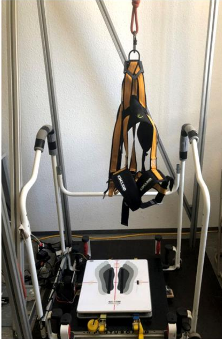
Fig. 2 Balance set-up with Posturomed, force-platform, and safety belt.
