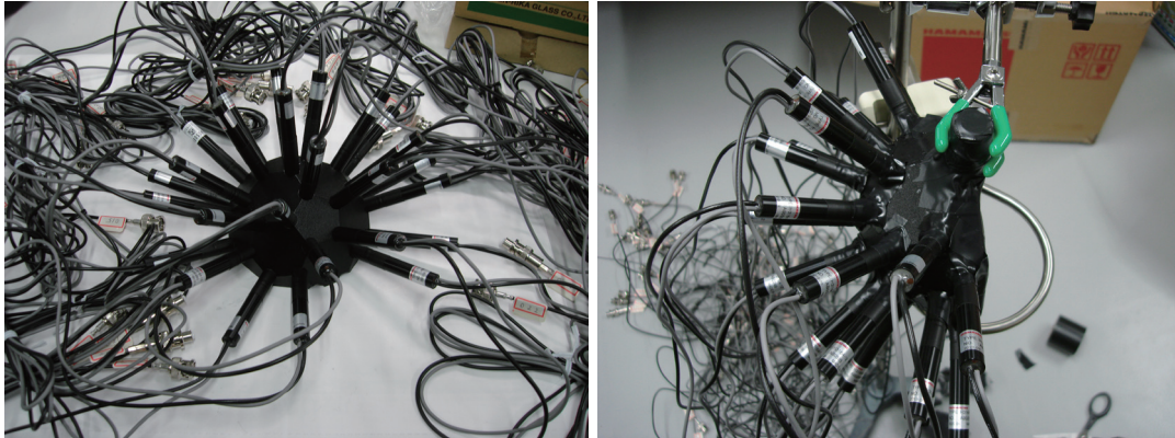
Figure 3. Left side panel shows the photograph when all PMT were mounted on the jig, and right side panel shows HUNI-ZICOS detector which consist of hemisphere flask adapted on the PMT mounting jig. In this time, we inserted UV cut filter between the flask and all PMTs in order to avoid the detection of scintillation from Anisole.
