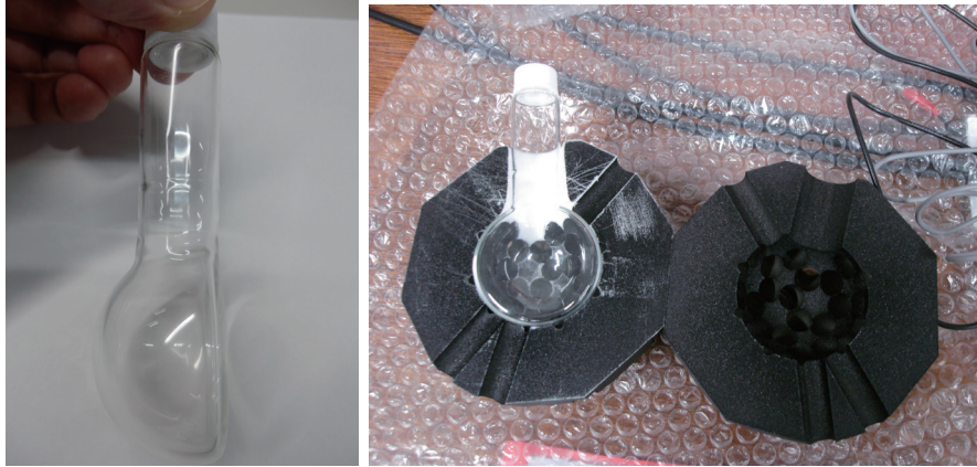
Figure 2. Left side panel shows the custom made hemisphere flask. The diameter is 50 mm, and the plastic screw cap was prepared in order to avoid evaporate Anisole. Right side panel shows the truncated icosahedron PMT mounting jig which has holes at each vertex.
