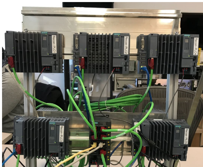
Fig. 15. Shipboard resilient control experimental system.
