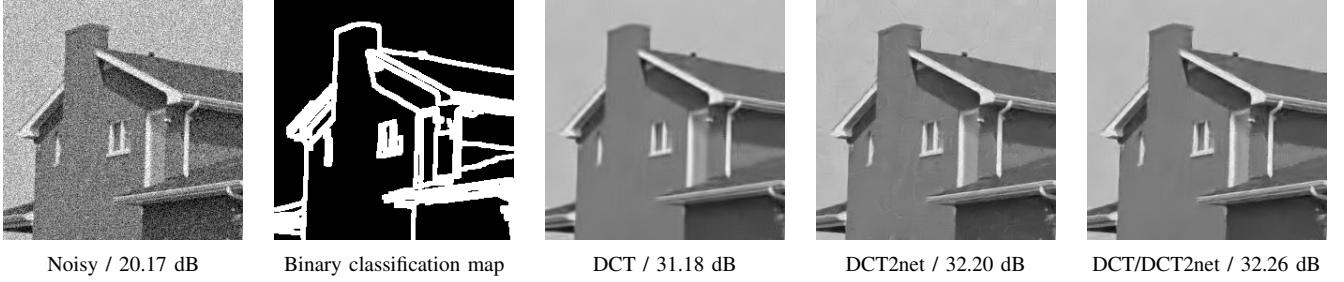
Fig. 8. Application of the proposed procedure to get a partition of the noisy image House . Pixels belonging to white areas after classification are denoised with DCT2net and the others with a traditional DCT denoiser. Results (in PSNR) are given for each method for a noise level \sigma = 25 .
