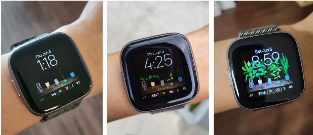
Figure 5.7: An example of a glanceable visualization on smartwatch’s watch face. In this watch face app called “Sprout,” the growth of the plants is mapped to the user’s step count. The plants reset daily.
