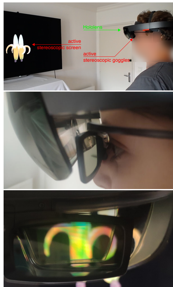
Figure 4: A user simultaneously wearing active stereoscopic goggles and an OST-HMD. At the top, an overview of the system in use. At the center, a close view on dual display wearing. At the bottom, the right user's eye view.
