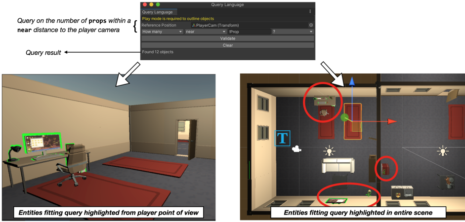
Fig. 9. Here we show the window to construct a simple query (Section 4.3) that counts the number of props within a near distance (3 meters) of the player camera. The two views show the highlighting in the scene from the player viewpoint (left) and the Unity scene view from above (right). The query and highlights can help the designer understand the real-time UX, and provide suitable guidance.
