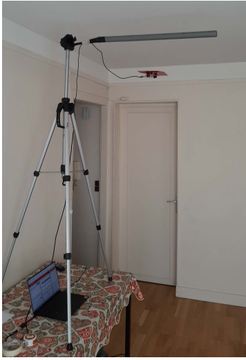
FIGURE 7. BOOSTXL-AOA angle of arrival estimation test setup.
