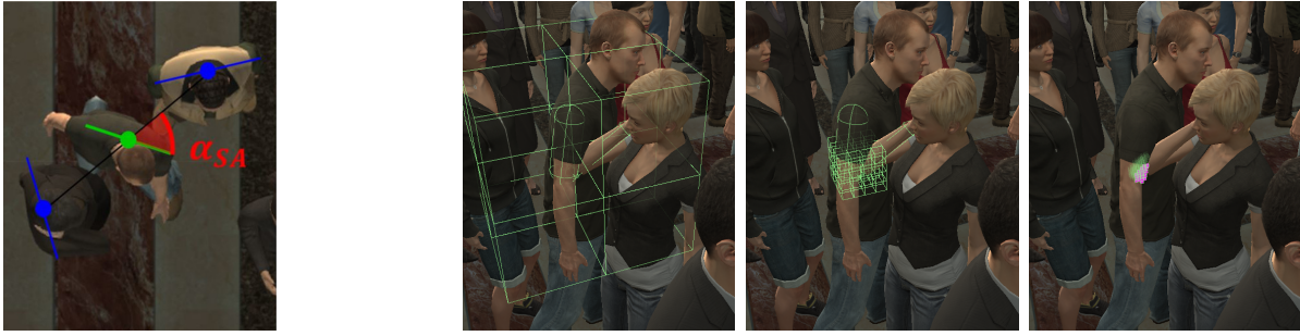
Figure 4.4: Left: shoulder rotations (angle \alpha_{SA} ) are defined between the participants’ shoulder-to-shoulder axis and the segment connecting the two virtual characters. Right: the volume of interpenetration is computed for each frame iteratively using voxel spaces of decreasing dimensions. The final interpenetration volume is displayed in purple.
