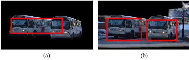
Figure 2: Ground truth pixels alone (a) are not always a sufficient amount of relevant pixels for a CNN to make good predictions (red box is inaccurate, misses second bus); contextual pixels at similar depth levels are also needed (b) for CNN accuracy (two good detections).
