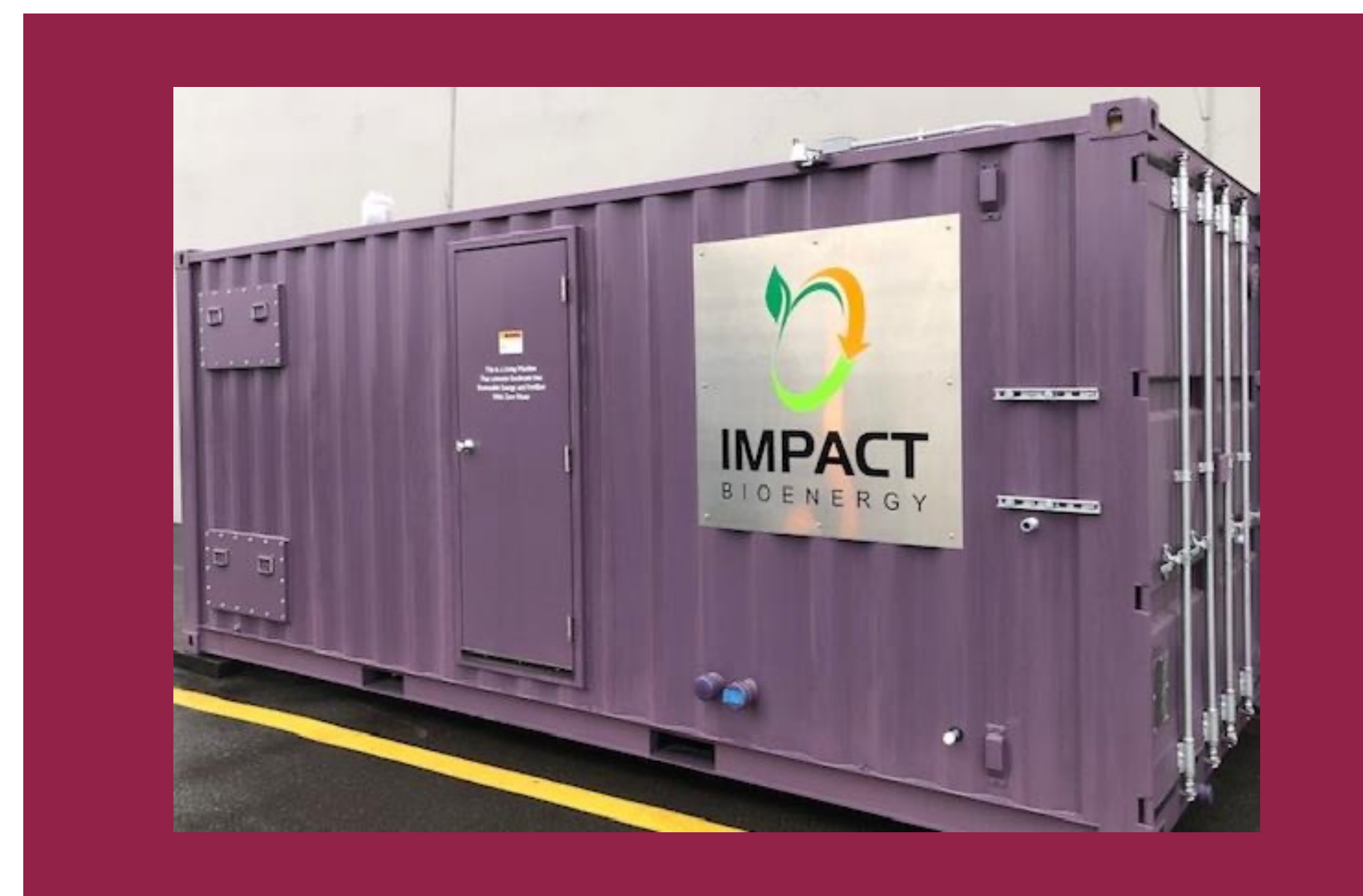
Figure 2. Impact Bioenergy High-solids Organic-waste Recycling System with Electrical Output Anaerobic Digester 25 (HORSE AD25). 11 The HORSE AD25 provides a scalable solution to food waste – converting it into liquid digestate and biogas.
