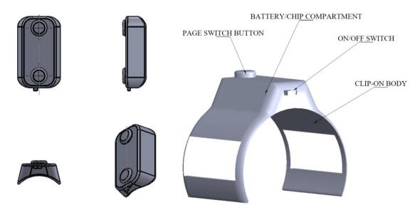
Fig. 1 First Designs of Instrument-Based Device
