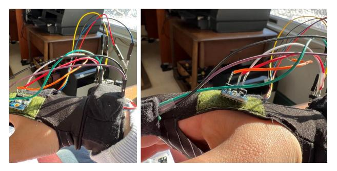
Additionally, these images show the high-winding nature of the wires; the system is not contained, and jumper wires with female heads have been used for trouble-shooting and testing.
