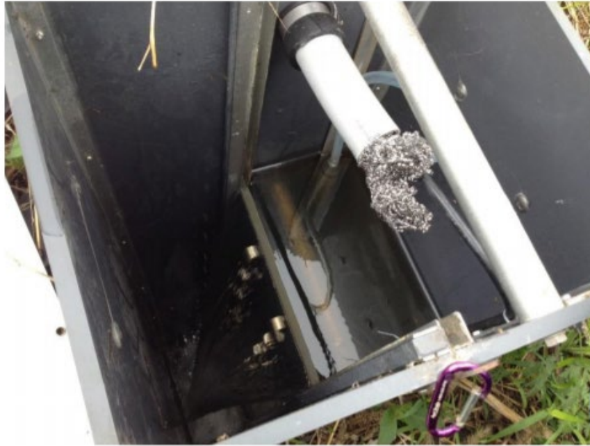
Fig 1. 7 AgriDrain weir box outlet structure for HHM, from [34]
