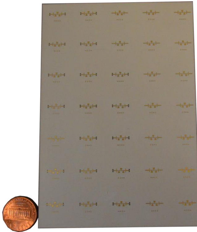
Figure 47: Manufactured panel section featuring 35 LCP lowpass filters
