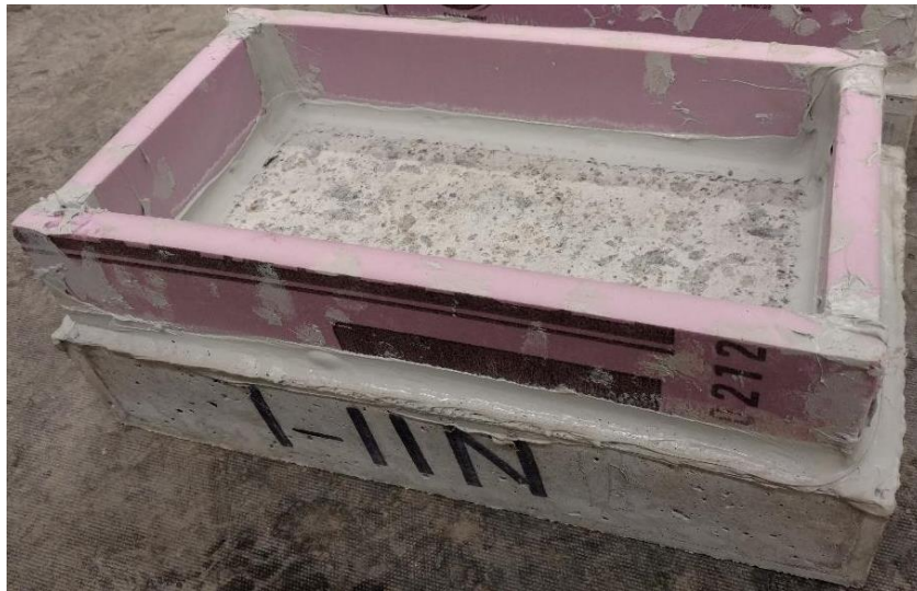
Figure 3.1: Scaling resistance test specimen
