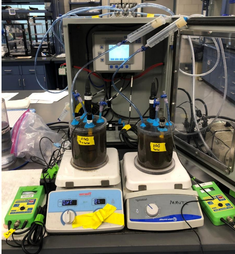
Figure 5: 1.2L Polycarbonate Sealed Reactors with YSI 5500D Multi DO Optical Monitoring and Control Instrument Set Up for Nitrification Max Rate Test.
