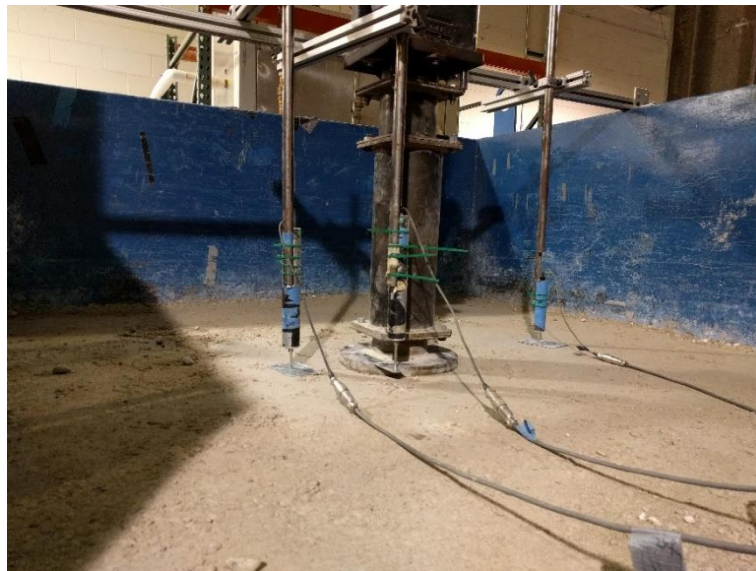
Figure 3.26. Surface of Base Course During Unpaved Test Sequence.
