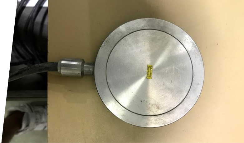
Figure 3.30. Earth Pressure Cell Used in This Study.
