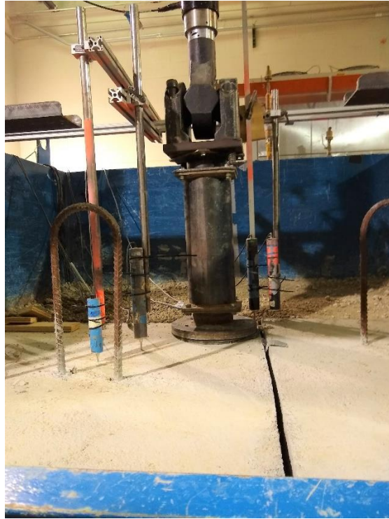
Figure 3.27. Displacement Transducers on Concrete Pavement Test.
