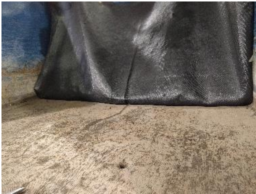
Figure 3.14. Woven Geotextile (after RAP Test).
