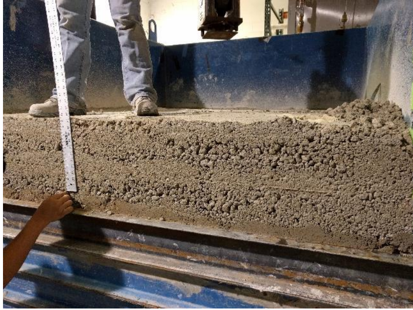
Figure 3.18. Direct Measurement of Base Course Thickness Post-Test.
