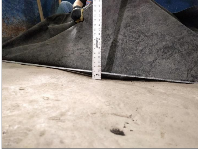
Figure 4.6. Subgrade Surface of the RAP/NW Section after Loading and Excavation.
