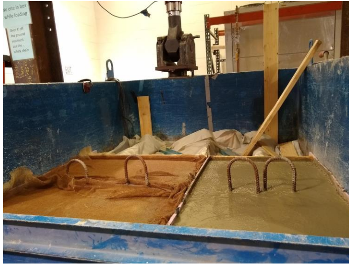
Figure 3.24. Concrete Slabs After Pour with Burlap Overlying to Preserve Moisture.
