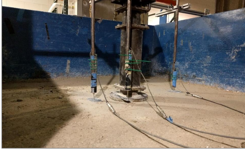
Figure 4.24. Surface Depression on the RCA Section after Cyclic Loading.
