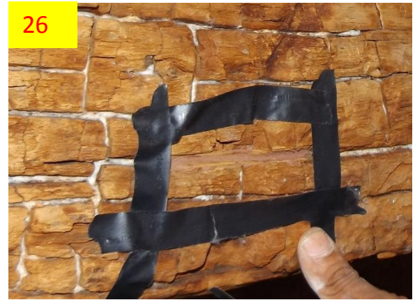
Photo 23-26 Injection by using B72 20 to harden the cotton, consolidating wood by using Plexisol P550 3-5-7% and making a test of filling on the cotton by using microballoon with a suitable color mixed with B72 15%
