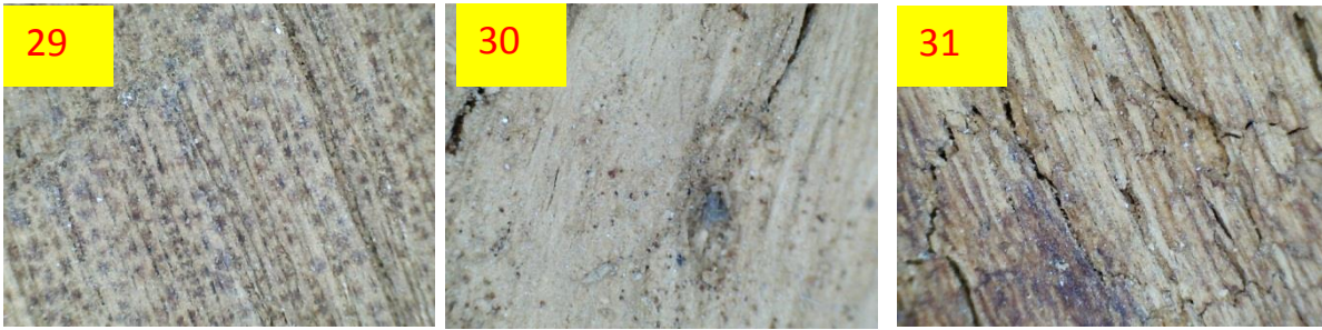
Photo 29-31 Digital microscope of the surface of the wood after mechanical and chemical cleaning
