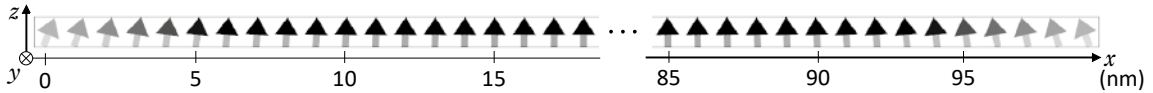
Fig. 7. Simulation results of MMs in the one-dimensional wire with D = -3.0 \times 10^{-3} \text{ J}\cdot\text{m}^{-2} . The direction of MMs near the edges is indicated with arrows.
