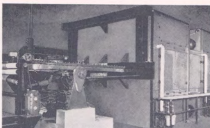
The Hunter VapoJet Tenter Dryer employs high-velocity super-heated steam, propelled through scientifically-arranged telescoping nozzles in close contact with the fabric. It achieves the ultimate in even drying and assures complete freedom from migration problems. Applicable to any tenter frame.
