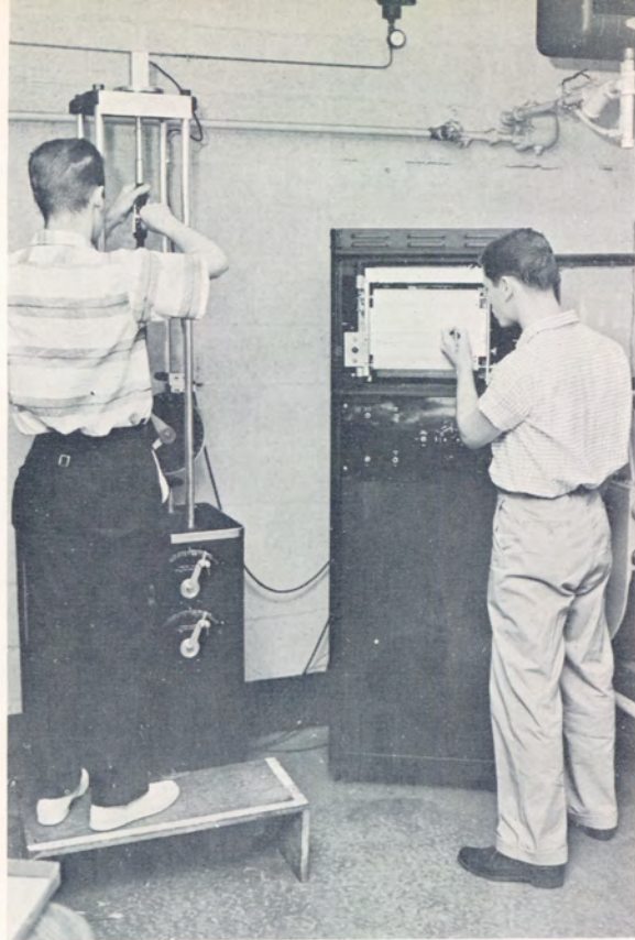
Physical Testing laboratory is equipped with instruments to measure strength, abrasive resistance, water and air permeability and other essential tests.
